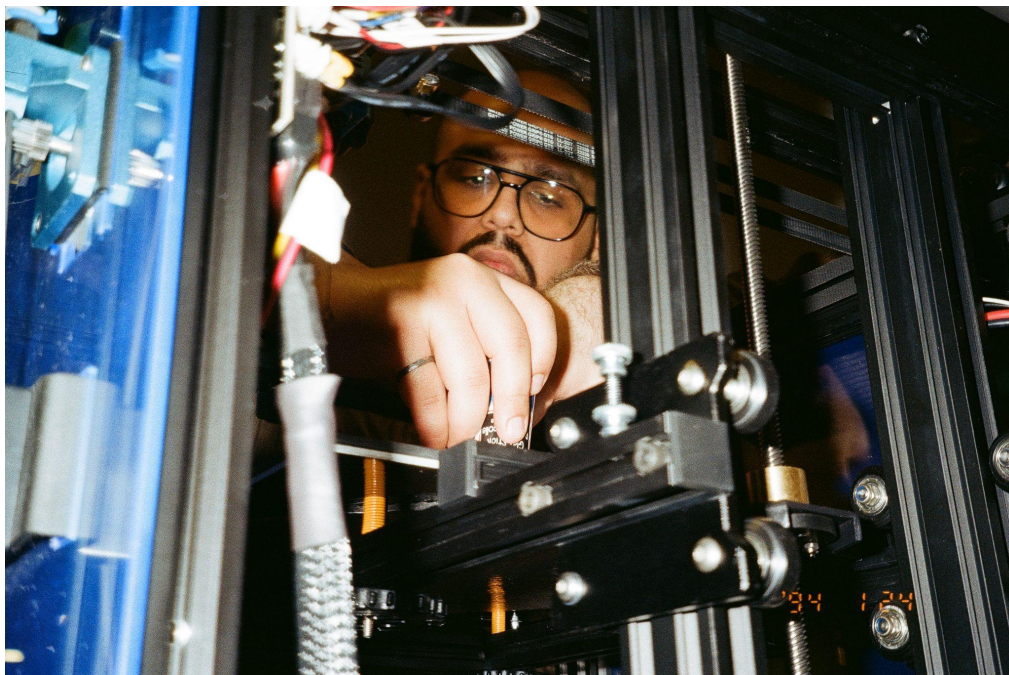
Figure G-10: Girish applying glue to the print bed for better adhesion.
