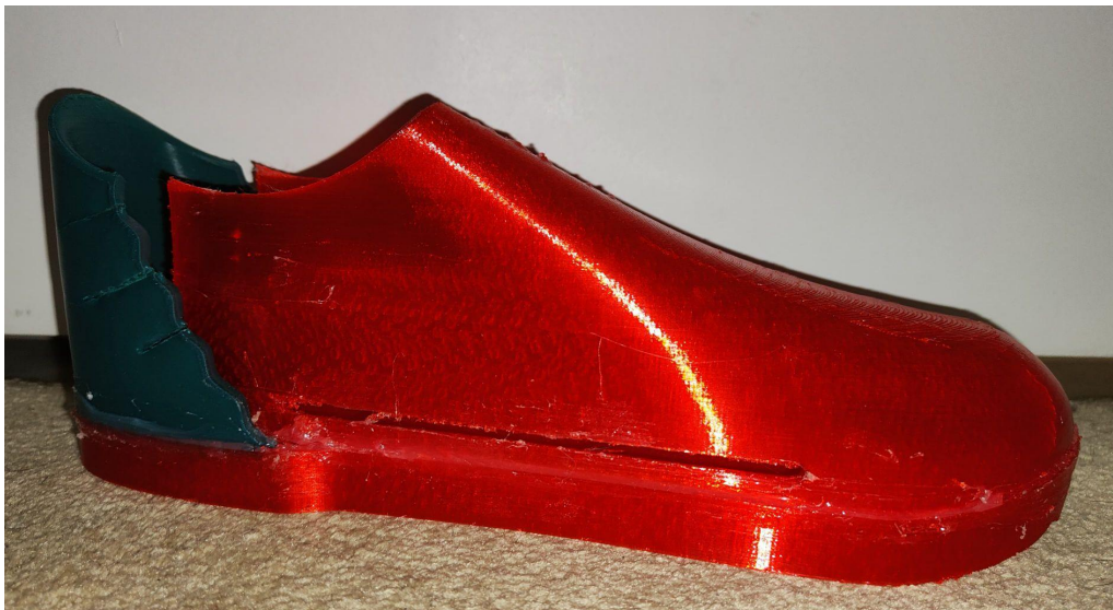
Figure 13.2: The shoe bonded by silicone caulking and using final prototypes.
