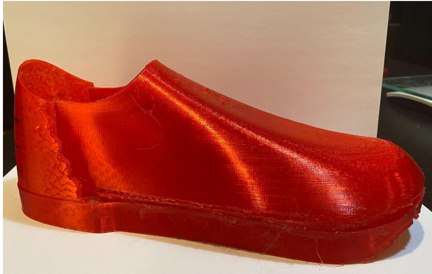
Figure 13.1: The shoe bonded by Gorilla Glue and using primary prototypes.
