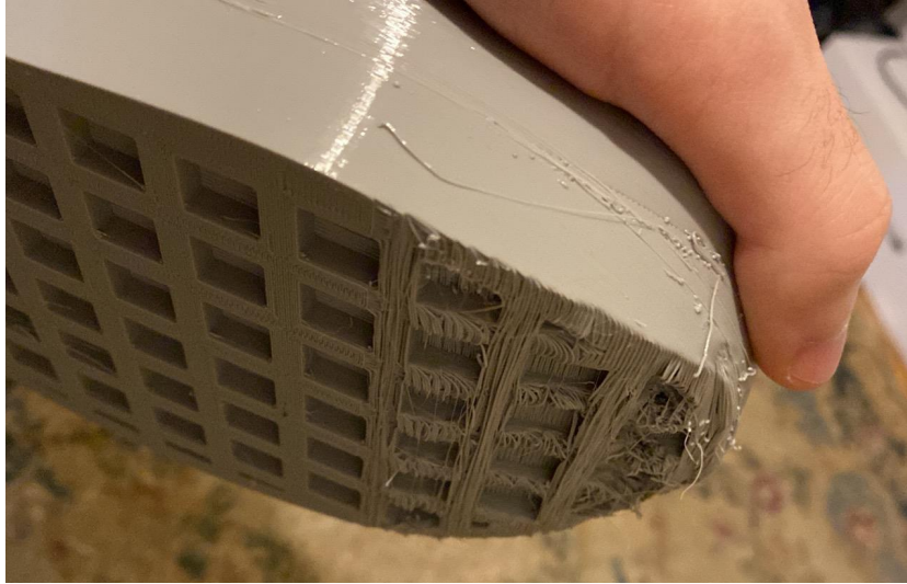
Figure 13.10: The print quality degrades at the toe area.
