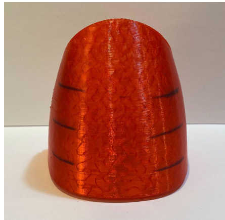
Figure 12.15: The first prototype of the heel with the suggested relief cut lines marked on the part.
