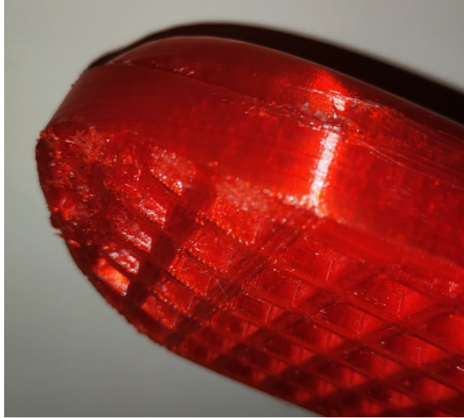
Figure 12.8: Improved toe box on the second midsole prototype.
