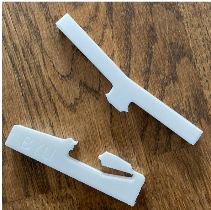
Figure 2.16: The compliant mechanism broke after only 33 cycles.
