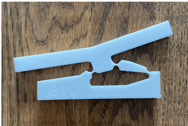
Figure 2.15: The printed bistable compliant mechanism.
