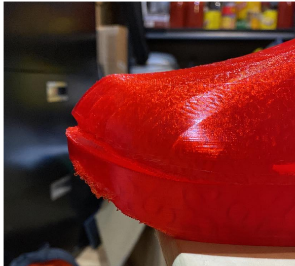
Figure 12.11: The slight gap between upper and midsole.
