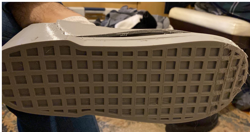
Figure 13.9: The width of the shoe is too small.
