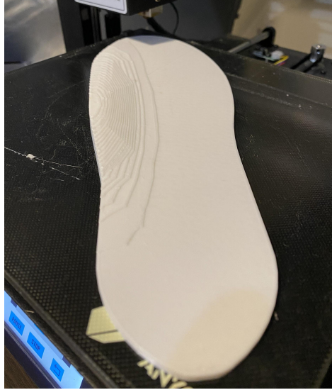
Figure 7.2: The first prototype print designed for fit testing.
