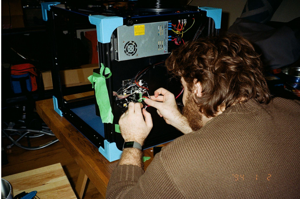
Figure G-13: Mahdi wiring in the printer motherboard.
